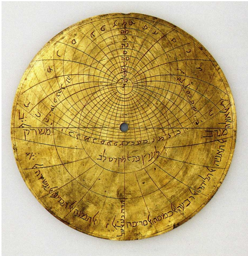
Fig. 5: The plate with markings for Jerusalem. Note that the peg at the top has been broken off so that the plate cannot be properly fixed inside the mater.
