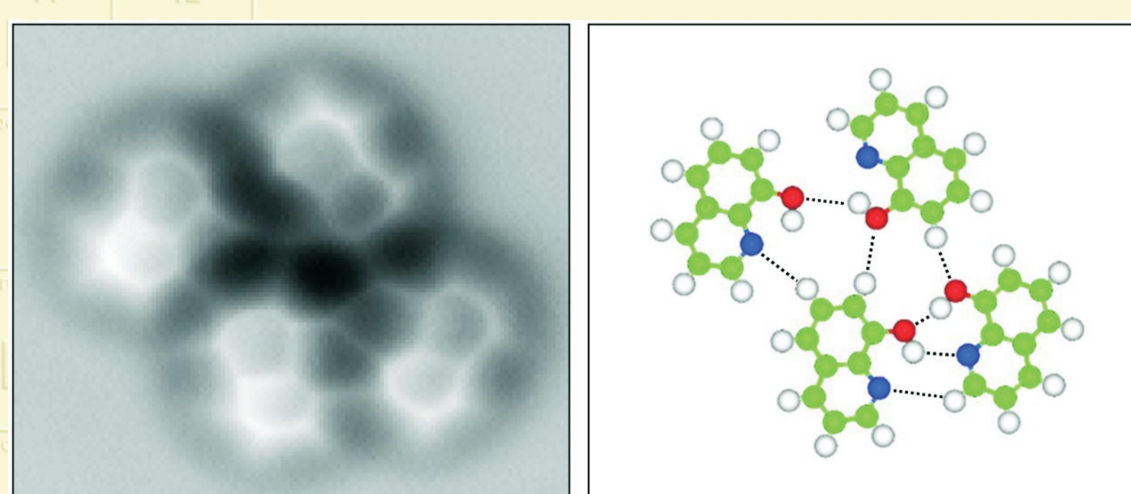
AFM images of 8-hydroxyquinoline on a copper surface shown hydrogen bonding interactions at room temperature. C=green; H=white; O=red; N=blue; Cu=orange
