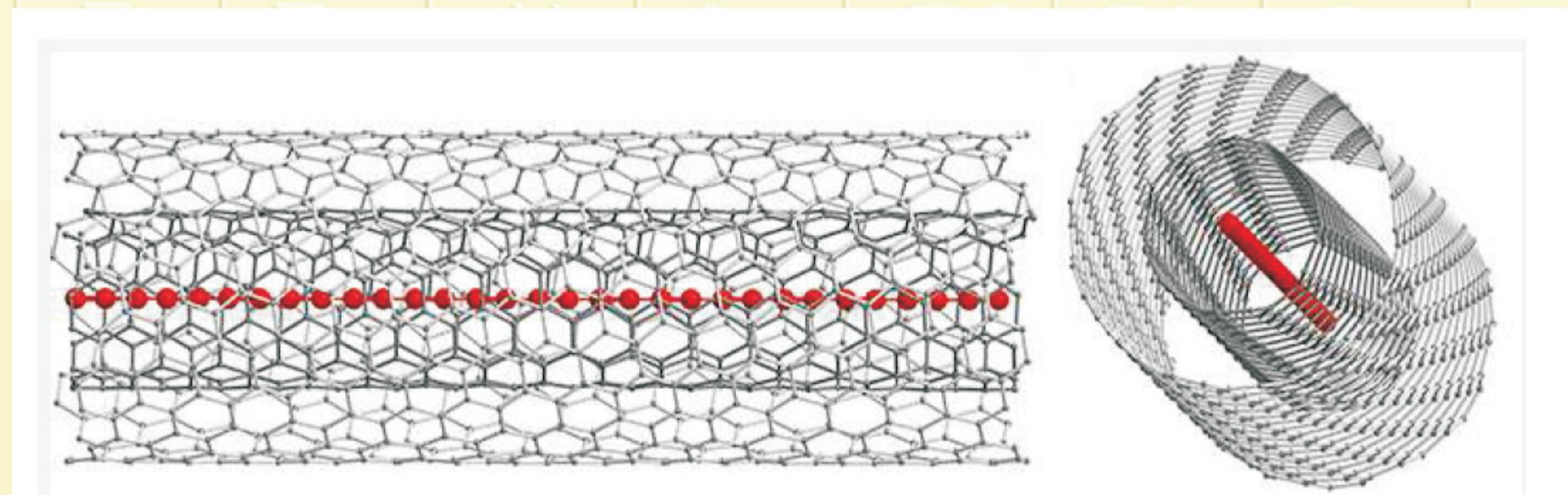
A long, linear carbon chain (red) resides within two carbon nanotubes (gray), as shown from two perspectives. The inner tube has a diameter of about 0.7 nm.
