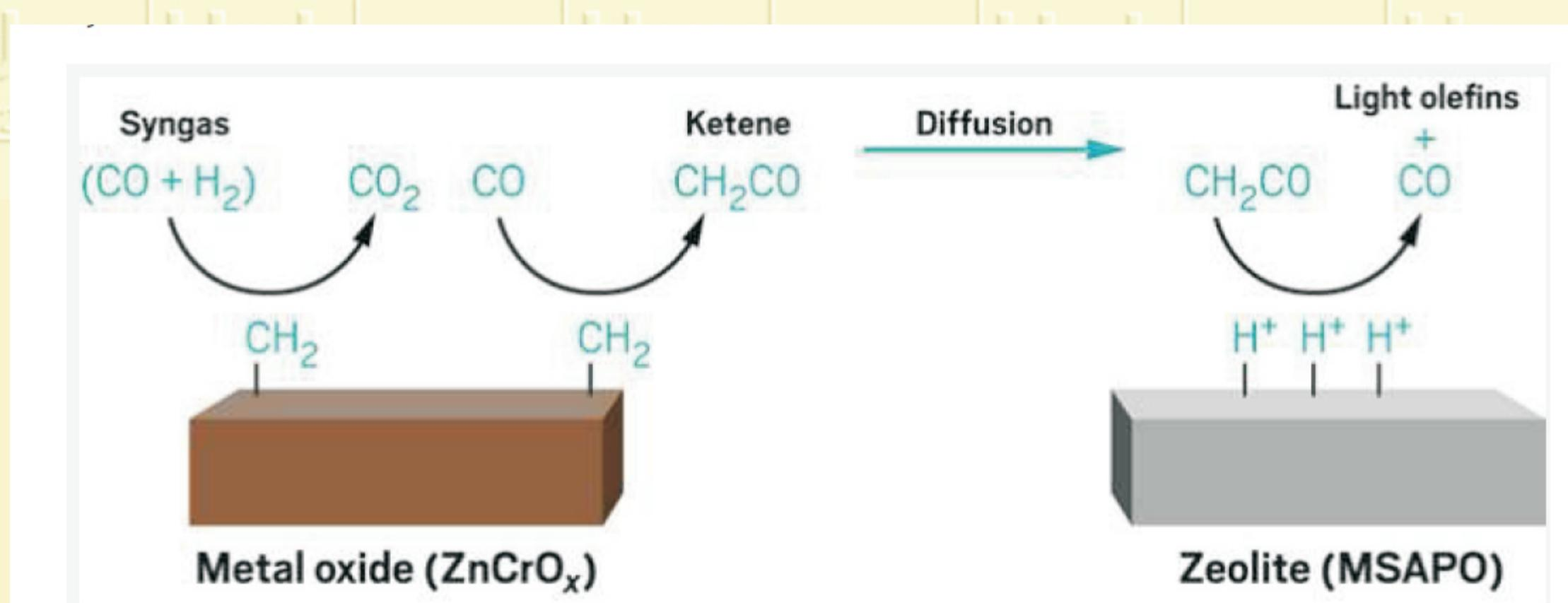
In the OX-ZEO technique, activation of syngas on a metal-oxide surface forms  $\text{H}_2$  groups that help create ketene, which then diffuses to a zeolite with hydrogen active site, giving rise to light olefins
