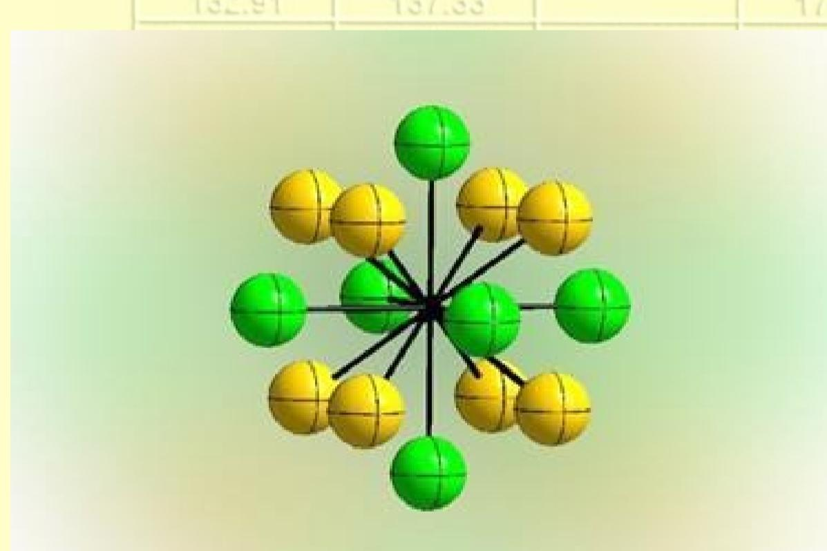
A section of the crystal structure of fluorine. The F1 atoms forming the cube are drawn yellow, the F2 atoms forming the octahedron are drawn in green.
