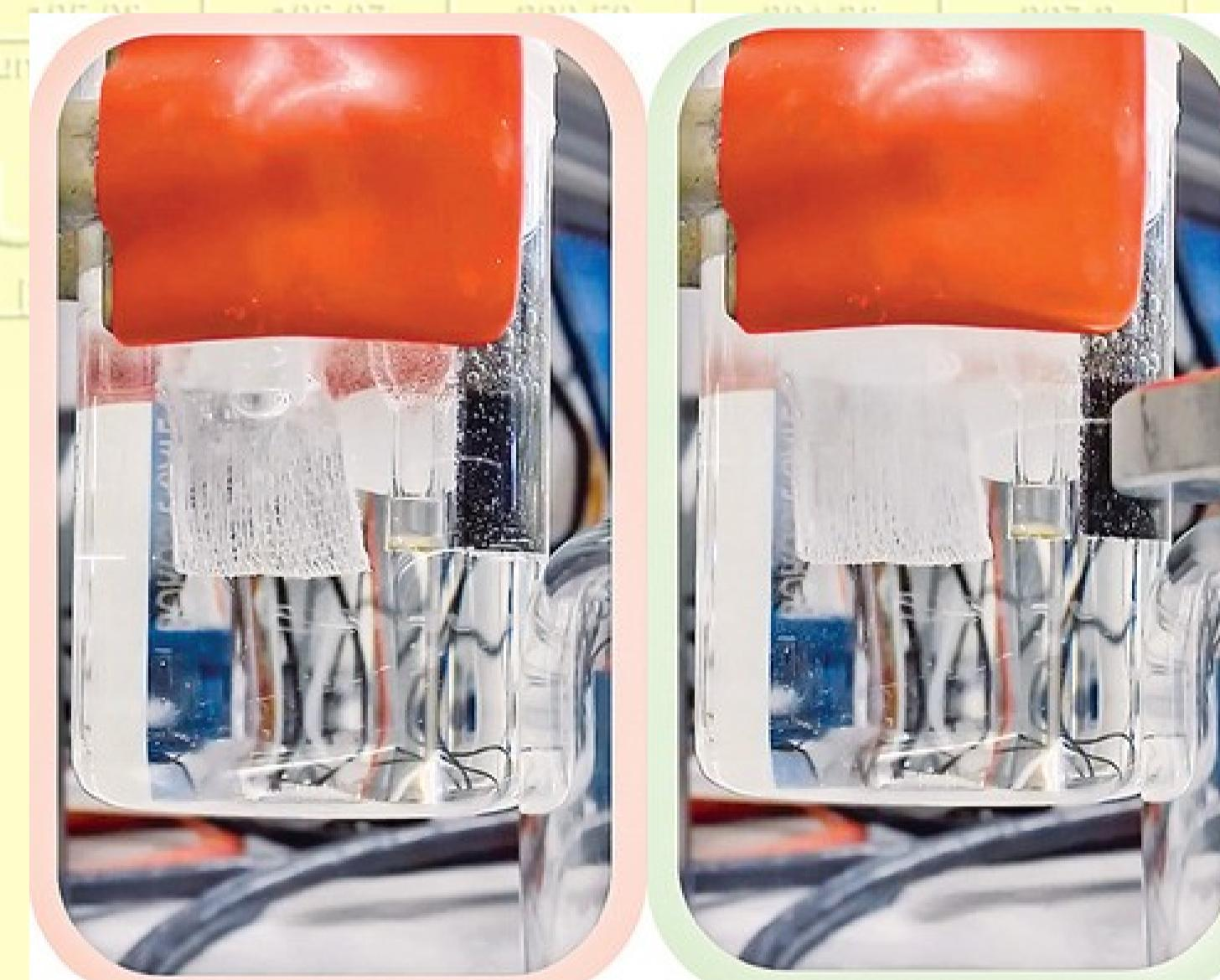
A gently bubbling electrolyzer (left) suddenly doubles its output of hydrogen and oxygen when a magnet is placed next to the anode (right), suggesting a simple way to make hydrogen more efficiently.
