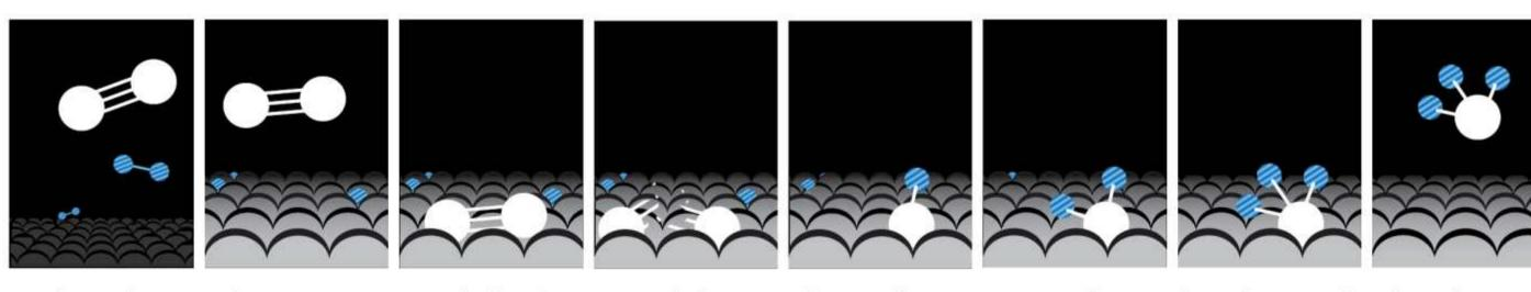
In the Haber-Bosch process nitrogen (white) reacts with hyrogen (striped) on an iron surface to then form molecules of ammonia which are released from the surface. This reaction, which extracts nitrogen from air, is an important step in the production of artificial fertilizer.
